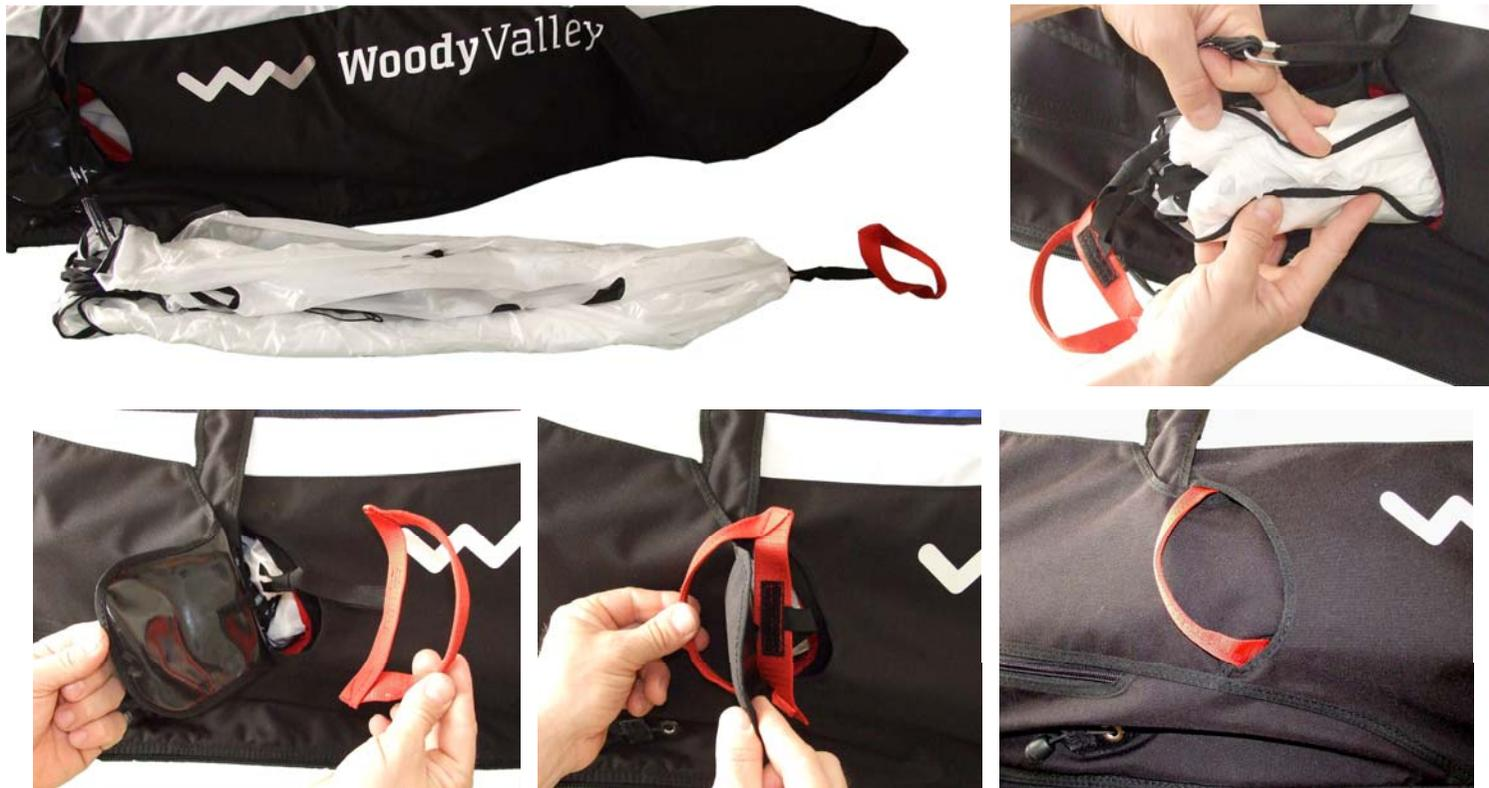
This system enables you to pull out your drogue chute and hold it in your hand during your approach to the landing field, launching it precisely at the desired moment. For immediate deployment, just release the handle immediately after extracting the drogue chute.
