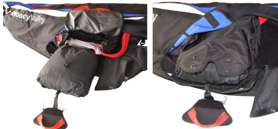
Insert a thin cord (1 or 2 mm diameter) into each elastic loop which will be used to close the housing. Using the cords, pull the elastic loops through the two smaller eyes, choosing those that best suit the size of your emergency parachute. Follow the order of closing the various flaps as shown in the drawings/photos below.
